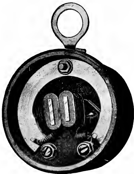
FIG. 59.—Interior view of a typical "watchcase" receiver.
